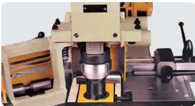
Punching equipment up to Ø 36 x 8 mm. in thickness
