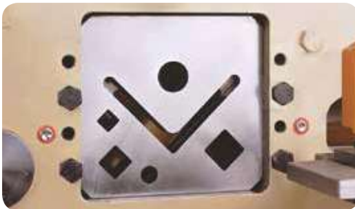
Ø and \square cut without deformation
