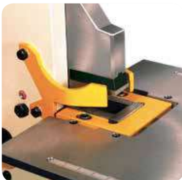
Rectangular notching with table. Bendicrop 50
